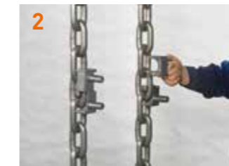
2 in das Kettenglied einschwenken have to be swiveled into the chain link
